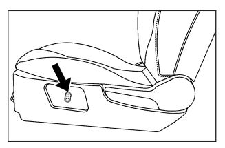
To adjust a power lift seat up or down:
